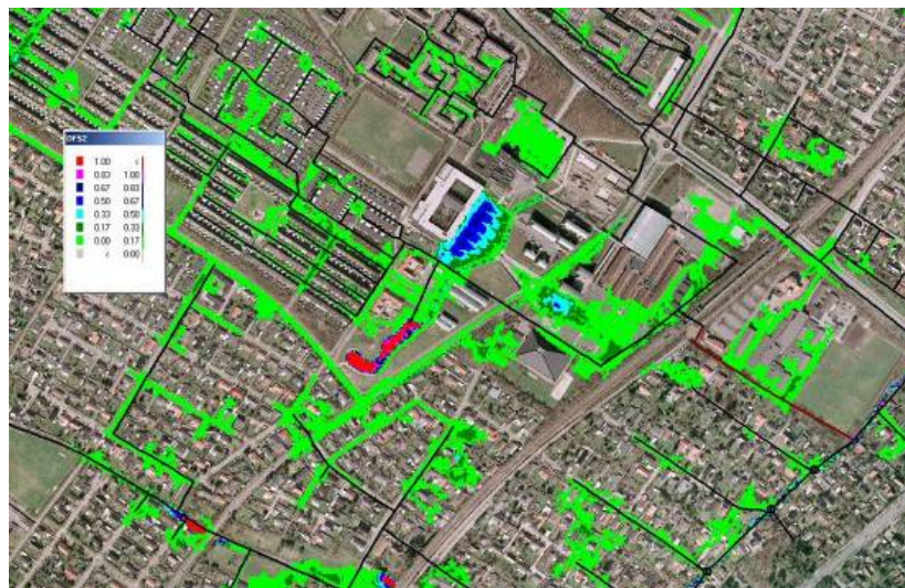
Flood depths computed for a future rainfall event with a 10 year return period. Climate Scenario: A2.
