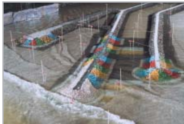
Verifying breakwater design with physical model tests.
